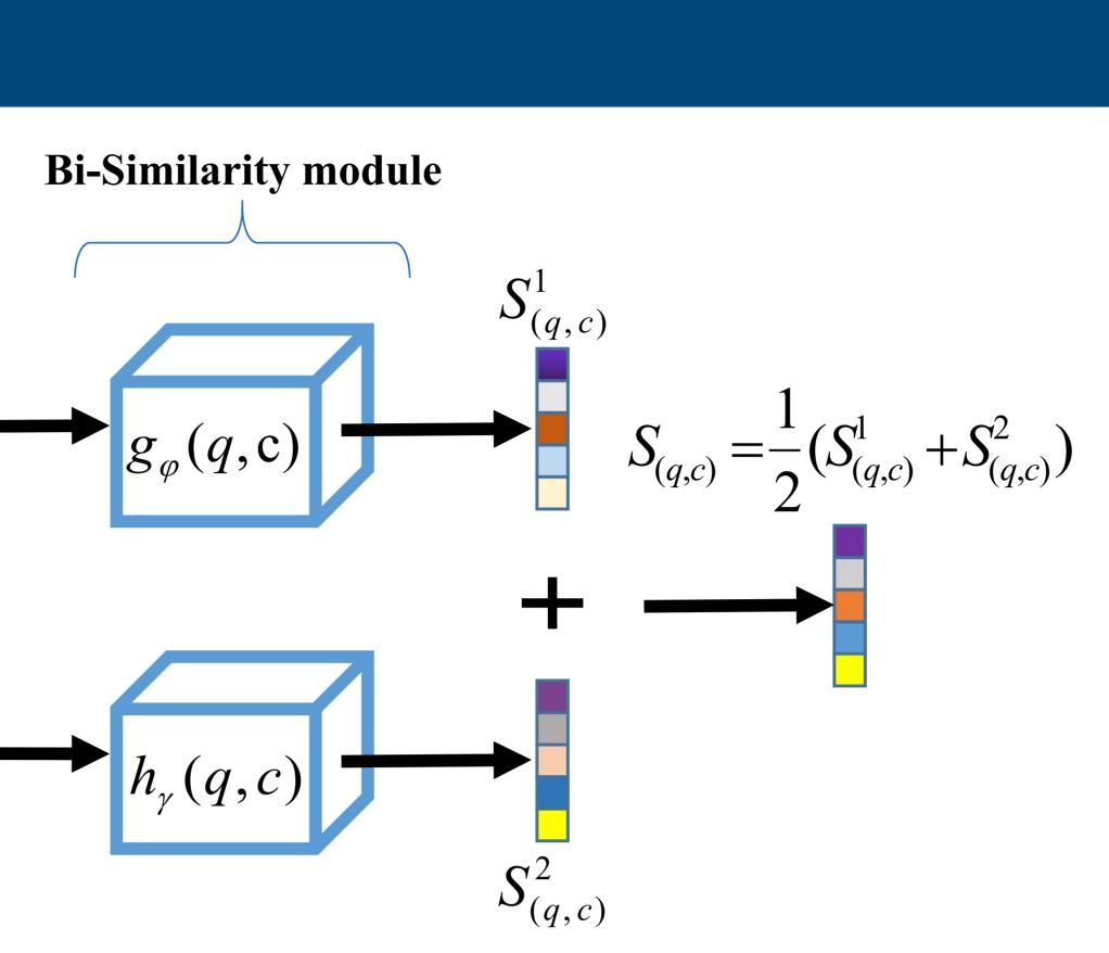
**Fig. 2:** Illustration of the proposed *Bi-Similarity Network* (*BSNet*). It consists of one embedding module  $f_{\phi}$ , followed by a bi-similarity module which outputs two similarity scores between a query image and C class prototypes in C-way K-shot problems.  $S_{(q,c)}^k$  denotes the kth similarity score between the qth query image  $x_q$  and the cth class in
